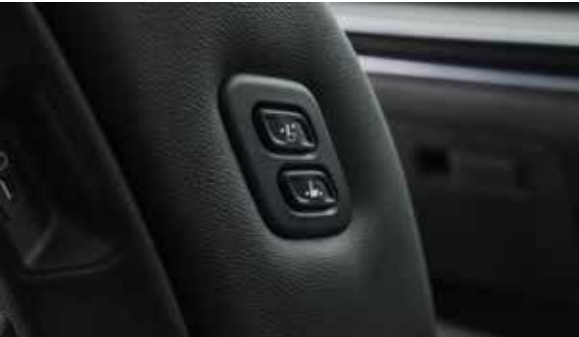
Passenger Walk-in Device With the press of a button on the inner side of the front passenger seat, the driver can temporarily move the seat forward and fold the seatback to let rear passengers in and out more easily.
