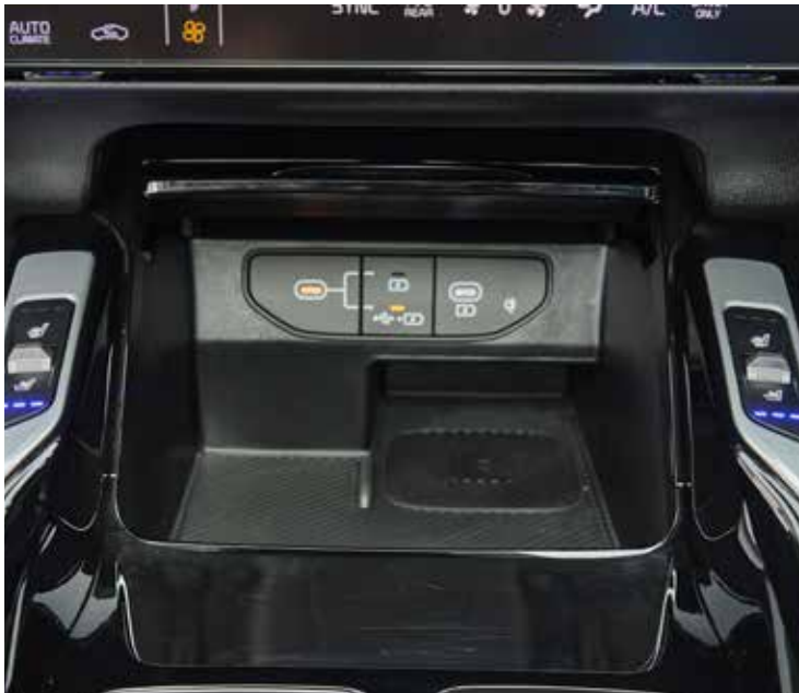
Wireless Charging Pad The rubber-lined, wireless charging pad in the center console can quickly charge compatible smartphones.
