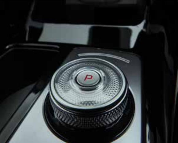
Shift-by-Wire (Dial Type) Features a Shift-By-Wire (SBW) system, offering seamless and effortless gear shifts with a modern, electronic rotary dial. This advanced technology enhances driving convenience, providing a smooth and intuitive transition between gears at the push of a button.
