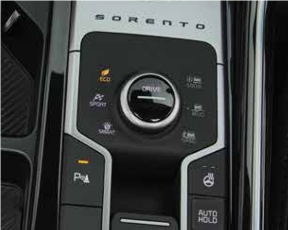
Drive Modes It offers multiple drive modes—Normal, Eco, Sport, and Smart—allowing you to tailor your driving experience to different road conditions.
