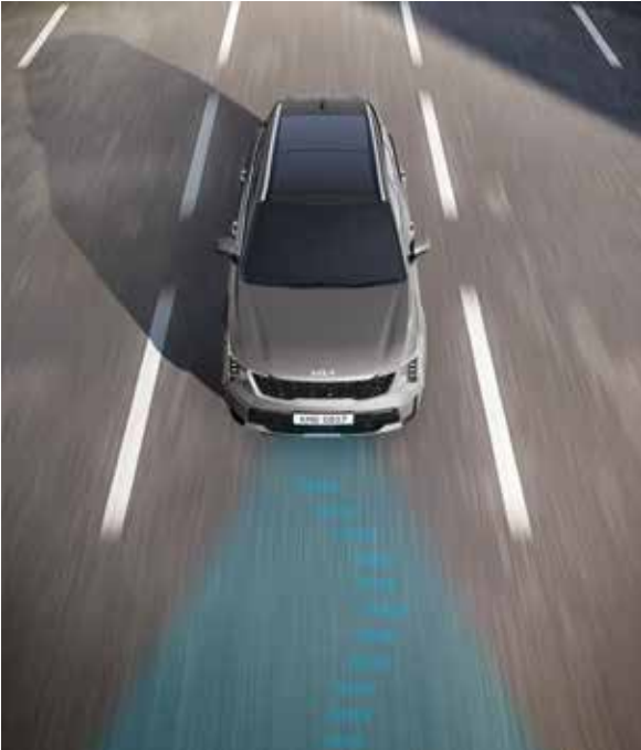
Lane Following Assist (LFA) To help you center the vehicle into lane while driving. LFA used the front view camera to help guide the steering based on lane markings or the car ahead.
