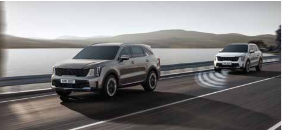
Smart Cruise Control (SCC) Smart Cruise Control (SCC, depicted above) helps you maintain a safe distance from the vehicle ahead at the speed you set. If the vehicle ahead stops abruptly, the Sorento automatically stops and then resumes acceleration.
