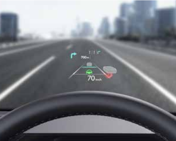
Colored HD Head-Up Display Keep your eyes on the road with the color head-up display projecting driving information within your field of view. The system displays alerts from the car's numerous driver assistance technologies, details of vehicle speed, and media.
