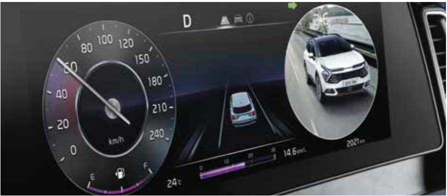
Blind-Spot View Monitor (BVM) BVM displays a rear side of the lane while changing lane. The image appears in the cluster to help maneuvering safely.
