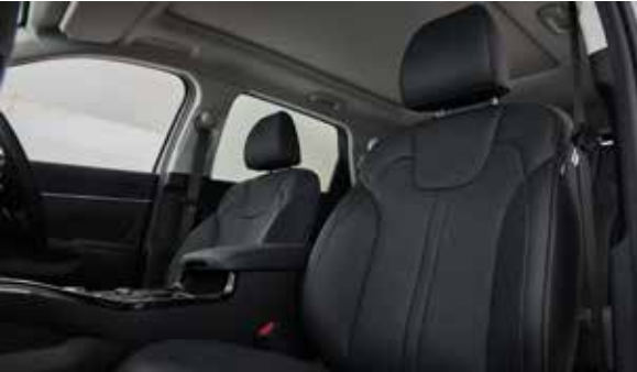
Ergo Motion Driver's Seat A system of air pockets means substantial support and comfort in a slim profile. The air pressure adjusts to match the driver's individual posture, with extra side support when in Sport drive mode.
