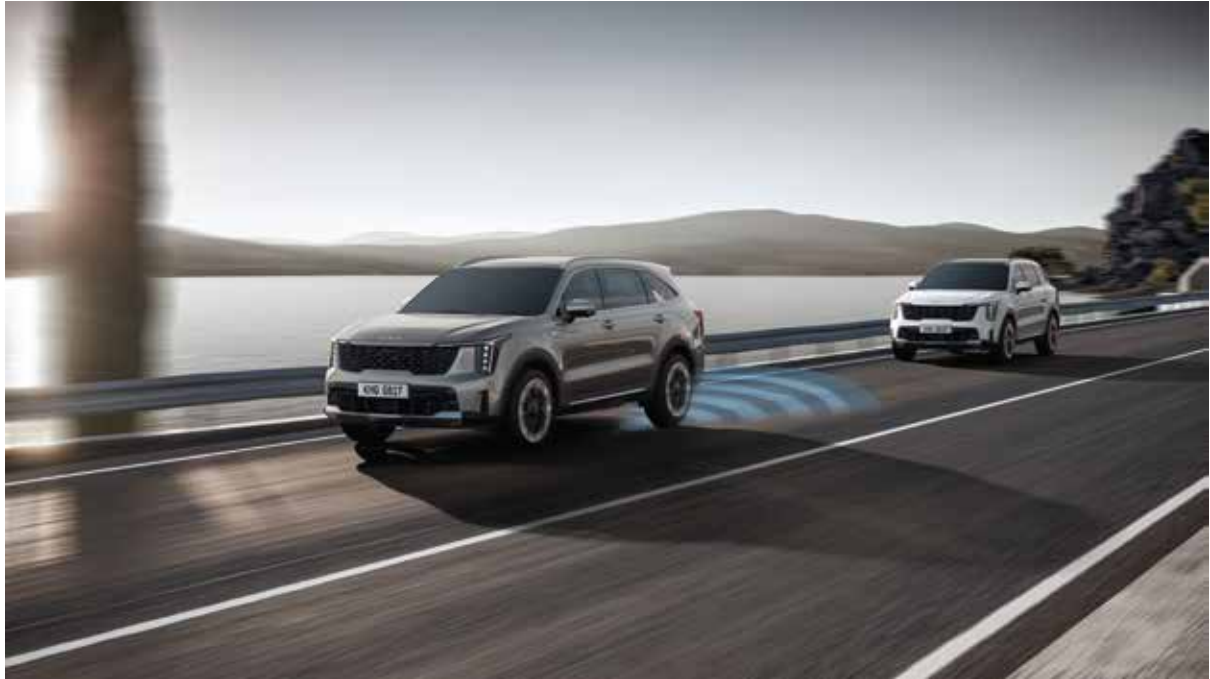
Lane Keeping Assist (LKA) Warns if a lane departure is detected without a turn signal switch operation. Automatically assists steering to prevent the vehicle from departing the lane only if a lane departure is detected without a turn signal switch operation.
