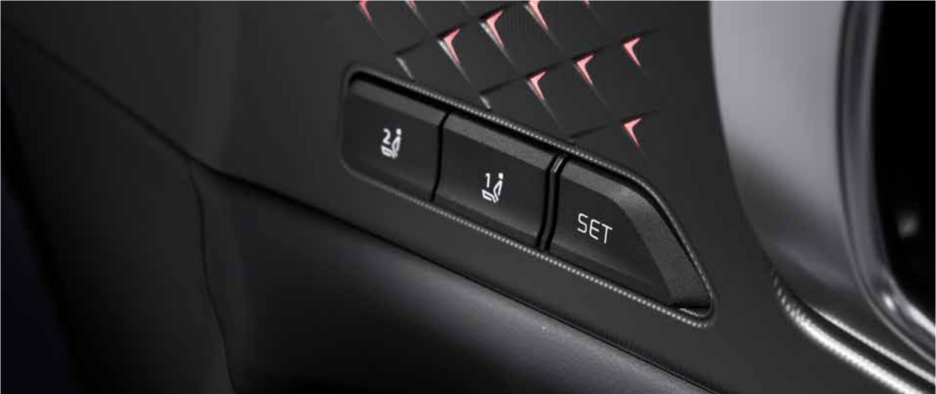
Integrated Memory System (Driver) The position of the driver's seat, side mirrors, and HUD can be memorized for up to two people and then recalled with a single-button operation.
