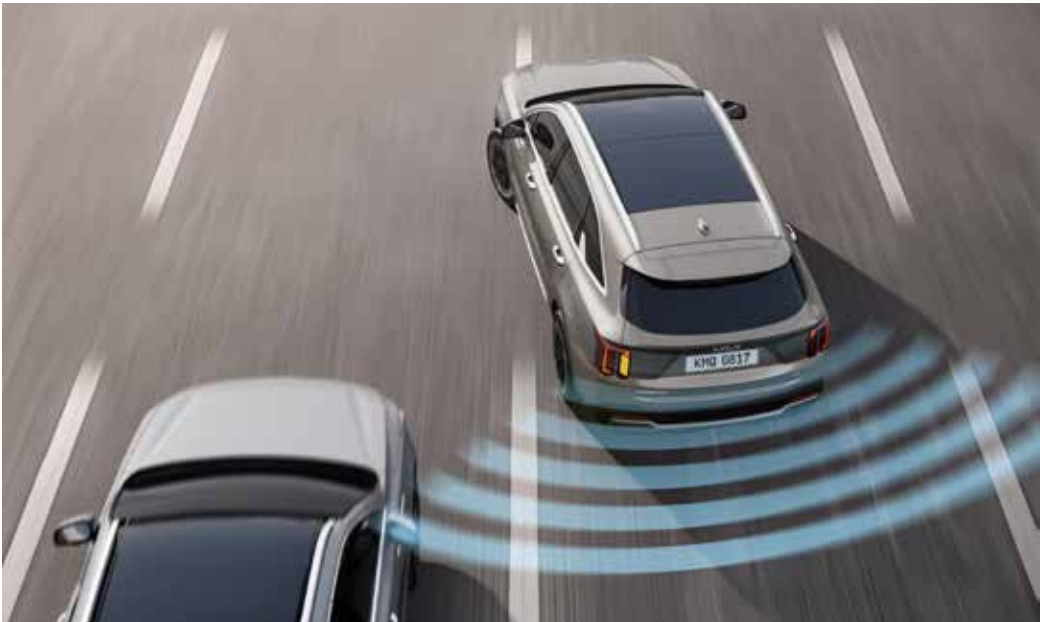
Blind-Spot Collision-Avoidance Assist (BCA) If you signal a lane change and BCA detects a risk of a collision with a vehicle approaching from the rear, it will automatically assist with braking to help avoid a collision.
