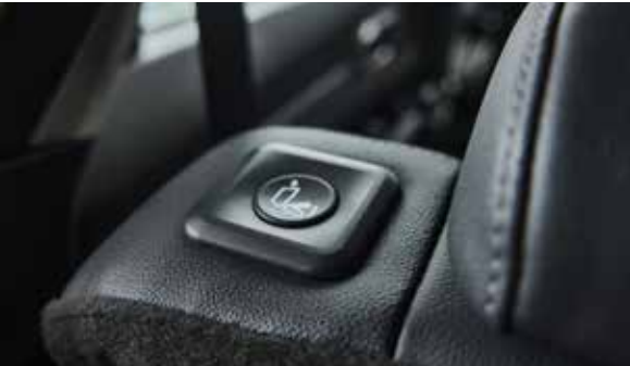
Smart One-Touch 2nd Row Sliding Walk-In Device This allows effortless access to the third row with a simple button press. This convenient feature automatically slides and folds the second-row seat forward, making entry and exit easier for passengers.
