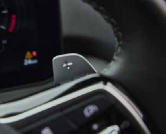
Paddle Shifters Located behind the steering wheel, paddle shifters allow drivers to easily switch gears without using the brakes and provide a sportier, smoother driving experience.
