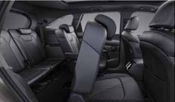
Smart One-Touch 2nd Row Sliding Walk-In Device This allows effortless access to the third row with a simple button press. This convenient feature automatically slides and folds the second-row seat forward, making entry and exit easier for passengers.
